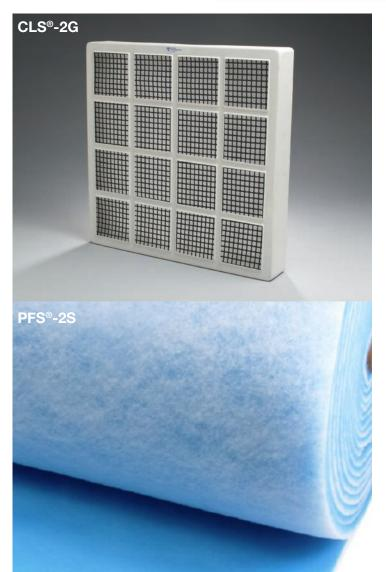
**CLS®** Coalescer / Prefilter media is available in synthetic or fiberglass pads cut to size to fit a 2" plastic frame. The prefilter combination is designed to remove the majority of airborne moisture and particulate mass prior to the air entering the TriCel® final filter.
