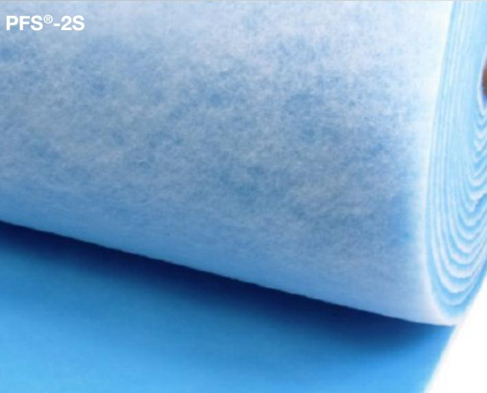
**CLS<sup>®</sup> Coalescer / Prefilter** media is available in synthetic or fiberglass pads cut to size to fit a 2" plastic frame. The prefilter combination is designed to remove the majority of airborne moisture and particulate mass prior to the air entering the TriCel<sup>®</sup> final filter.
